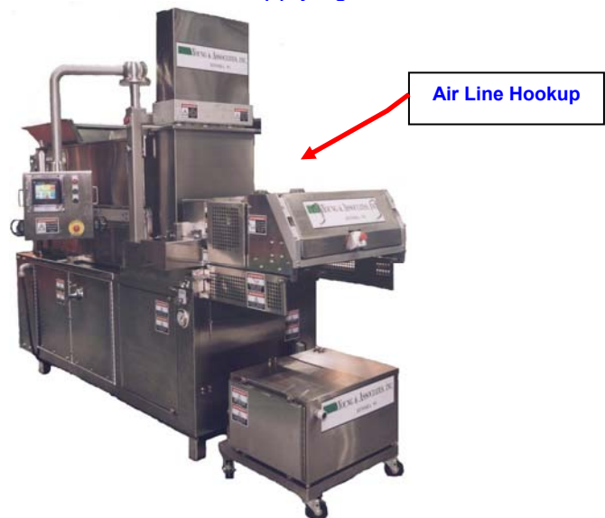
Figure 8: Paper Bar Blowback Air Line Hookup
